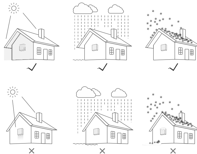
▲ Figure 4.1 Recommended Installation locations
